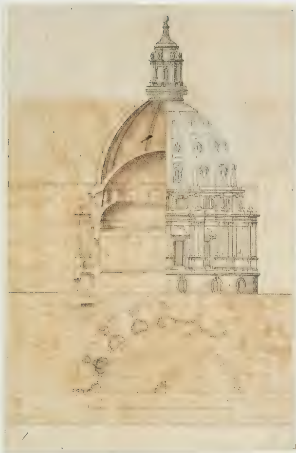
51. Revised design for the dome of St Paul's Cathedral, in four separate pieces, pasted onto a base sheet, by Nicholas Hawksmoor. c.1690 (section and plan), with reused elevation pieces from c.1687-88. Brown inks and pencil, 46.8 by 30.5 cm. (St Paul's collection, Guildhall Library, London; KD 95).
