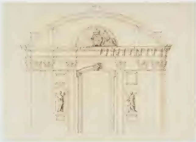
48. Elevation of revised central bay, north transept front, St Paul's Cathedral, by Nicholas Hawksmoor. c.1687-88. Brown ink and pencil, 31.2 by 43 cm. (St Paul's collection, Guildhall Library, London; KD 10).
