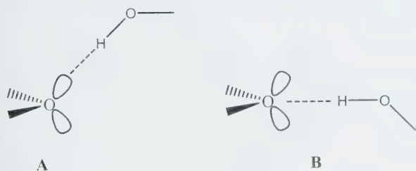
Fig. 1. The two possible structures of the 1:1 complex of an ether (or peroxide) with a hydrogen bond donor as proposed in ref. 3.
