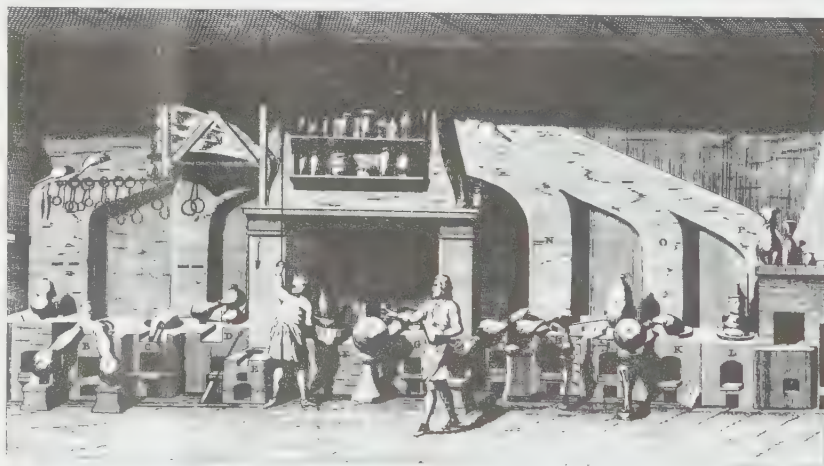
This "View of Practical Chemistry" from the April 1751 issue of the Universal Magazine depicts a variety of sand baths and other furnaces set up for distillations, extractions, and related operations. The accompanying discussion, third in a series begun in 1747, provides instruction on "the power of fire upon bodies, and the method of regulating it, so as to produce the desired effect." From the E. F. Smith Memorial Collection.
