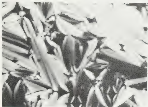
3. Smectic liquid: many Schiff's bases of terephthaldehyde look like this. 50x Photomicrograph Aldrich No. 12229-7
