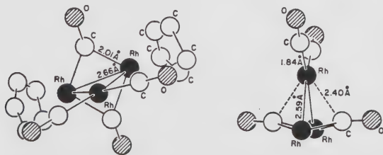
Illustration 6: Two views of the structure (in a crystal) of \text{Rh}_3(\text{C}_5\text{H}_5)_2(\text{CO})_4 .
