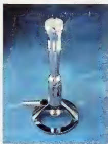
The Fisher burner, hailed as a major advance over the original Bunsen burner, has been a best-selling appliance for decades. A new version, the AccuFlame, lets researchers "fine tune" to any flame shape desired.
