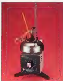
A workhorse in petroleum-testing facilities worldwide is this Fisher instrument for measuring the flash point of fuel and lubricating oils. It's precision-made to official specifications.
