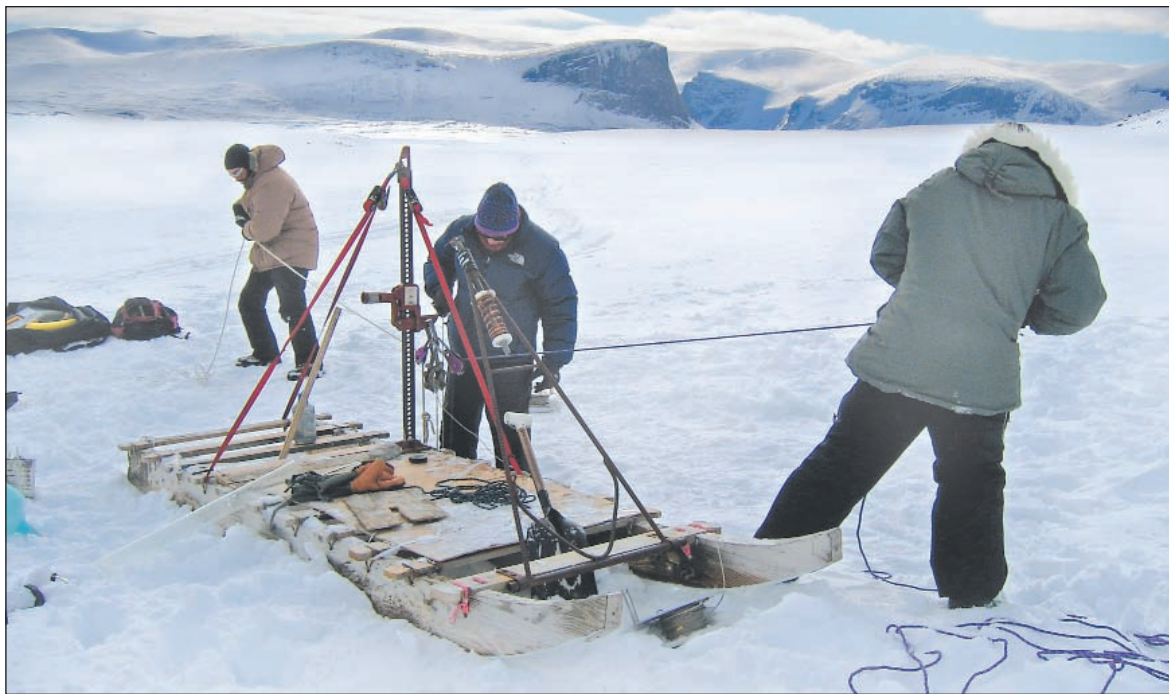
Using a sled-mounted coring system, researchers extract a sediment sample from a lake bottom on Baffin Island.
