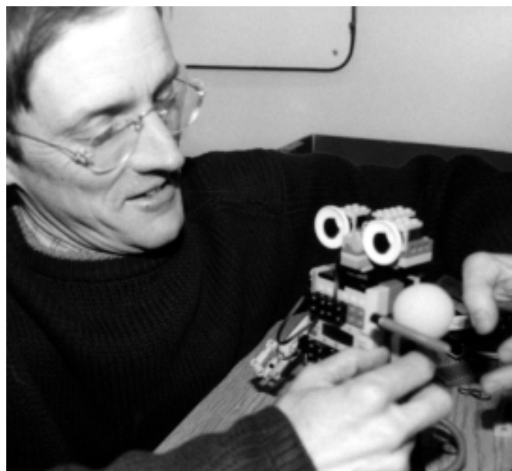
Ron Peterson with a Lego robot, created by an intern in the Department of Continuing and Distance Studies. The robot is programmed so when it shakes its right hand, it karate chops with the left hand.
