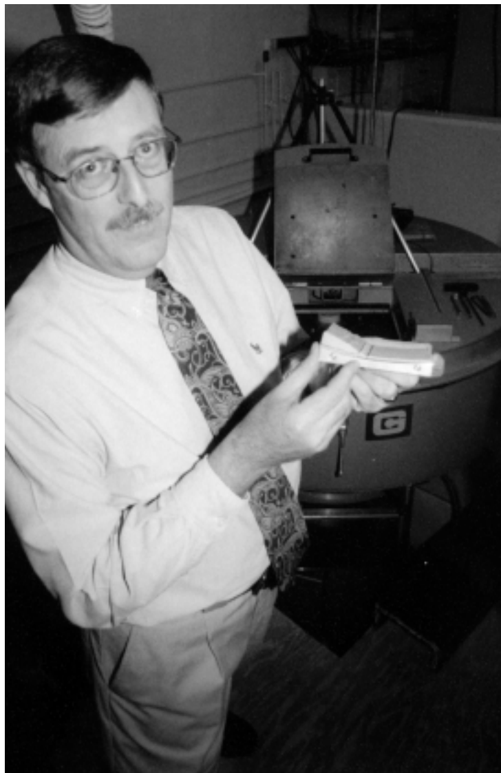
Geologist John Dixon displays clay model that he uses to explore the effects of plate tectonics on Rocky Mountain foothills. Centrifuge in the background acts like a time machine, helping researchers simulate the effects of gravity on the Earth's crust.
