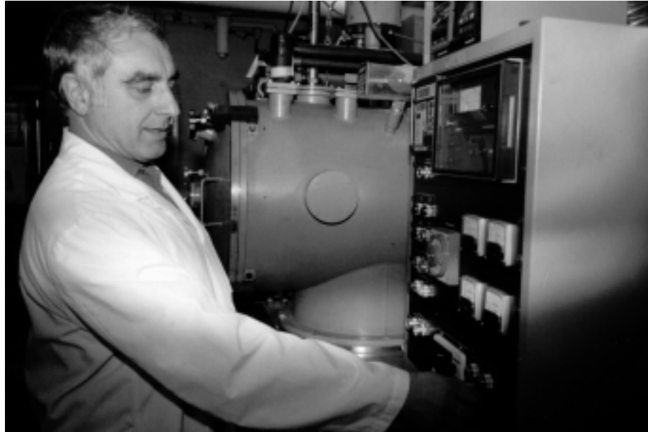
Vladimir Krstic monitors the high temperature sintering furnace in his lab in Nicol Hall.
