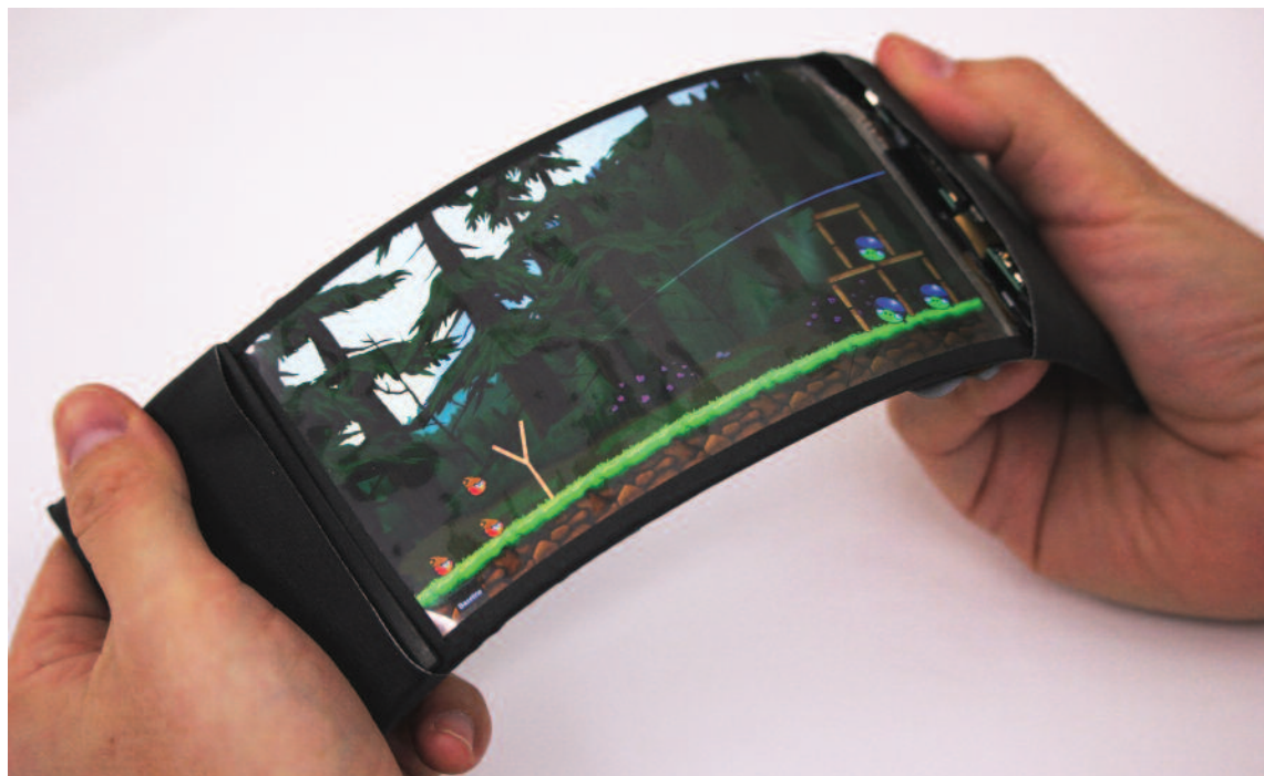
A user demonstrates how bending the ReFlex phone could be used in gaming applications. While playing the popular game 'Angry Birds,' the user sees the band stretched backwards as the phone is bent, while voice coils simulate the feeling of the rubber band being stretched.
