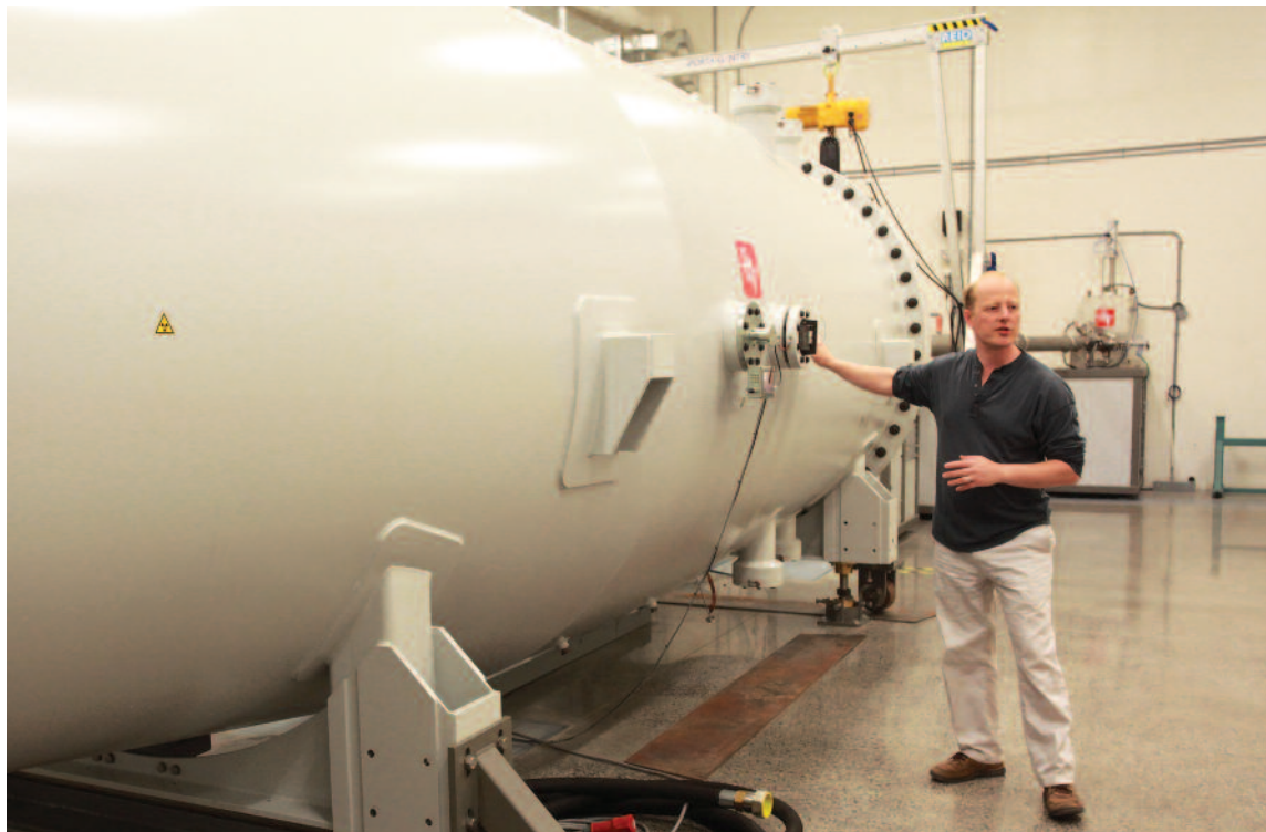
Mark Daymond (Mechanical and Materials Engineering) explains the high voltage tank that is part of the accelerator during a tour of the newly-opened Reactor Materials Testing Laboratory.
